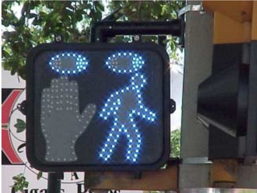
Figure 1. A photograph of an LED pedestrian WALK signal with an animated 'eyes' display to prompt sighted pedestrians to watch for turning vehicles.
